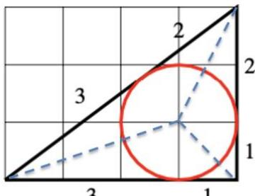
(1) Draw a 3-4-5 right-angled triangle on a grid. Using compasses construct the internal bisectors of the angles of the triangle and then draw the inscribed circle (we'll call it an incircle).
