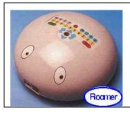
There are small toy robots with a pad of keys on their backs so that children can press keys for 0, 1, ...9 and keys for forward, back, right and left.
