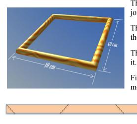
This stand is made from cylindrical wooden dowel of diameter 1 cm joined at the corners with 45 degree mitres.
