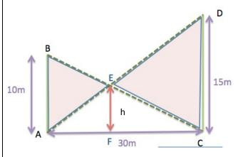
CF: FA is the ratio of the heights of  $\triangle$ CED and  $\triangle$ AEB so CF = 18 m and FA = 12m.  $\triangle$ AEF is similar to  $\triangle$ ADC so h/15 = EF/DC = AF/AC = 12/30 = 0.4 <u>Thus the height h = 6 m.</u> If the poles were distance d apart then CF : FA = 3 : 2 gives CF = 0.6d, FA=0.4d and AF/AC = 0.4 as above. Thus the height of E does not depend on how far the poles are apart.
